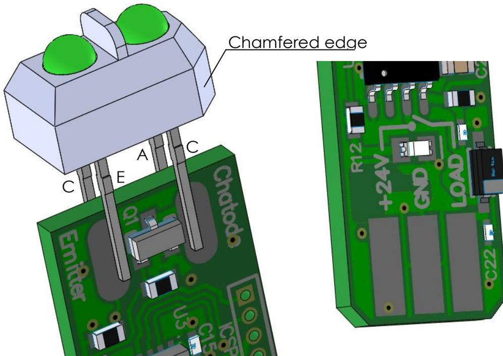
The power and output pads are situated on the opposite end of the PCB (+24V, GND, LOAD). A pin header or individual wires can be soldered on these pads.
